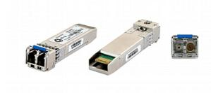
SFP1-SM-D is a fiber optic transceiver using 1310nm single-mode signals. These standard pluggable SFP optical modules have two LC connectors for reception and transmission over two strands of single-mode optical fiber
